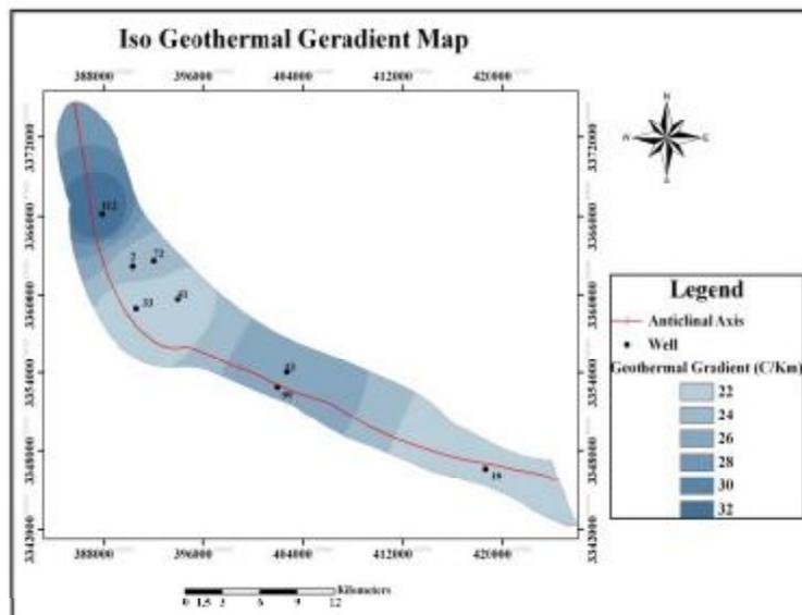
Figure 6. Iso geothermal gradient map of Rag-e-Safid oilfield (those wells that geothermal gradient of them is measured are also plotted).
