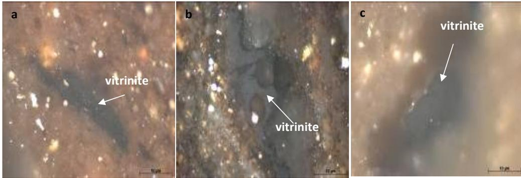
Figure 2. Digital image of some studied polish sections, a: well no. 18, Pd Fm, 2795 m; b: well no. 2, Kz Fm, 3392 m; d: well no. 33, Kz Fm, 2856 m.
